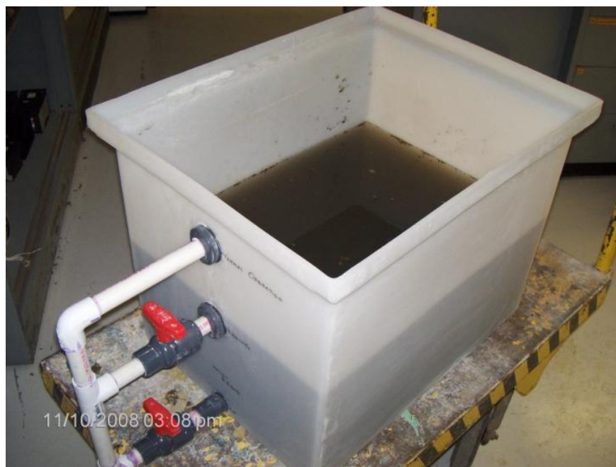
Figure 5.2: Initial aerated batch system mussel laboratory microcosm.
